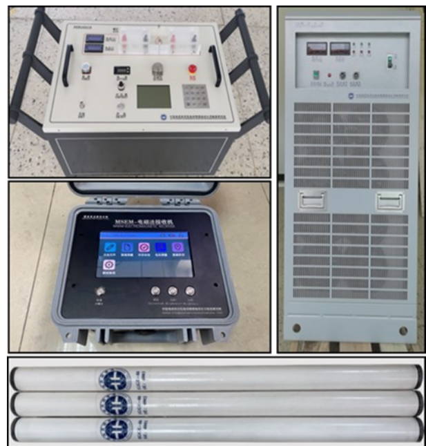
Figure 2. Multi-frequency CSEM system
