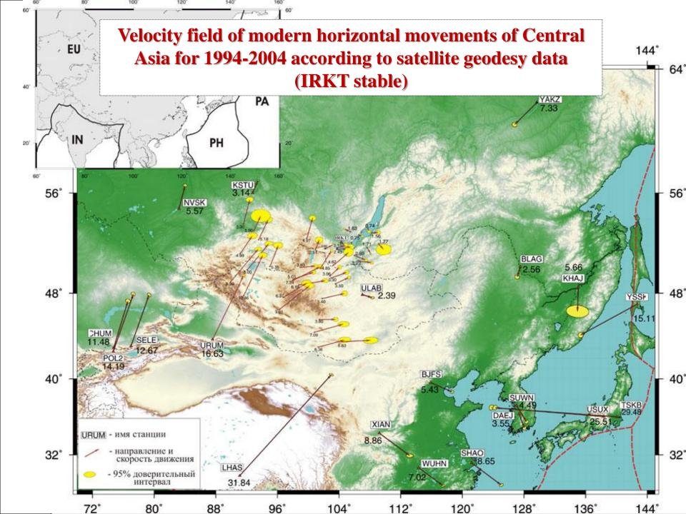
Velocity field of present day horizontal deformations of the earth's surface in the Mongolian-Siberian region based on satellite geodesy data (Lukhnev et al., 2010)
