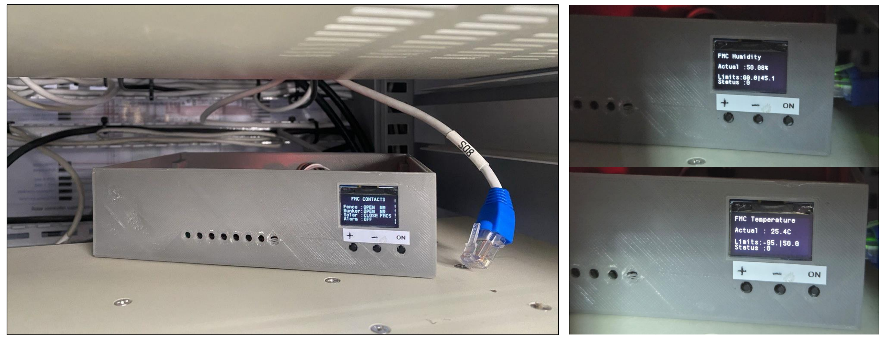
Figure 7. The OLED display in the station showed door status, temperature, and humidity
