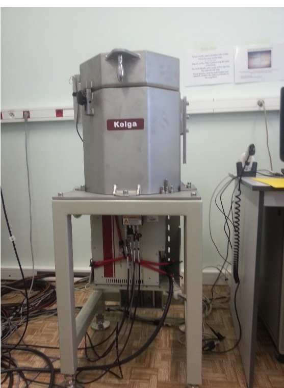
Canberra CP5 detector for Radionuclide measurement
