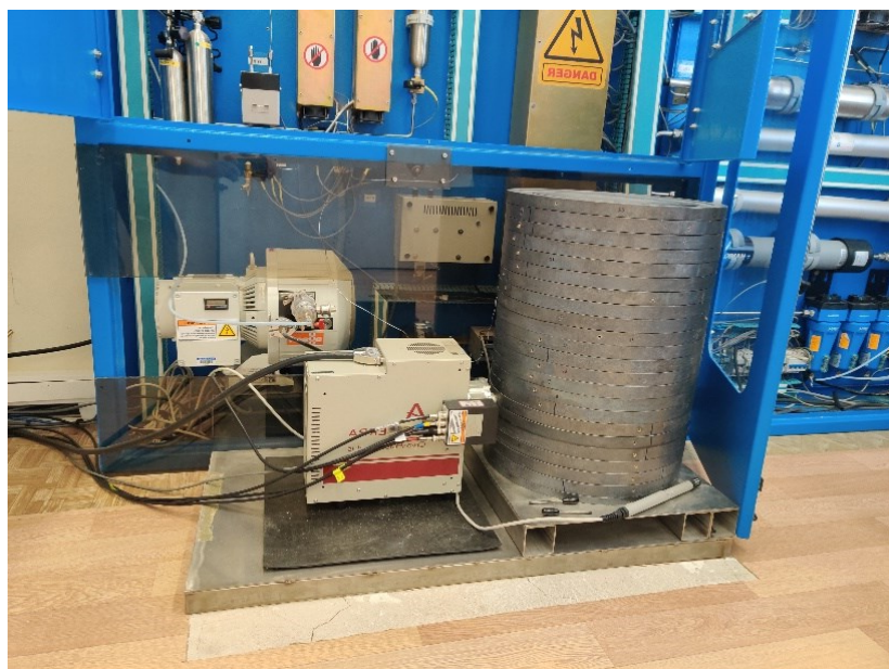
Canberra CP5 detector for Radionuclide measurement
