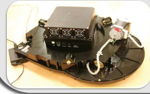
A chopper wheel is employed to maximize astrometric solutions in a single CCD frame, and a de-rotator is used to compensate field rotation of the alt-az type mount. The chopper can split the trail of the moving objects like asteroids and artificial satellites, and also record the time log when the chopper's blade block the time sensor. It makes a CCD image can have many streaks with their own time log. After data reduction, OWL can calculate the orbit of the moving object.
