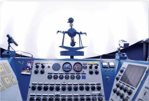
Image 1. Konica Minolta "MS-8" analog specialized device, control unit of the equipment.
