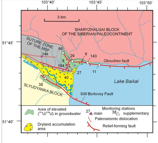
Location of station 27 and other main and supplementary stations for hydrogeochemical monitoring of active faults on the western coast of Lake Baikal (Kultuk area). Paleoseismic dislocations in the suture zone of the Main Sayan Fault (MSF) are shown after (Chipizubov, Smekalin, 1999).
